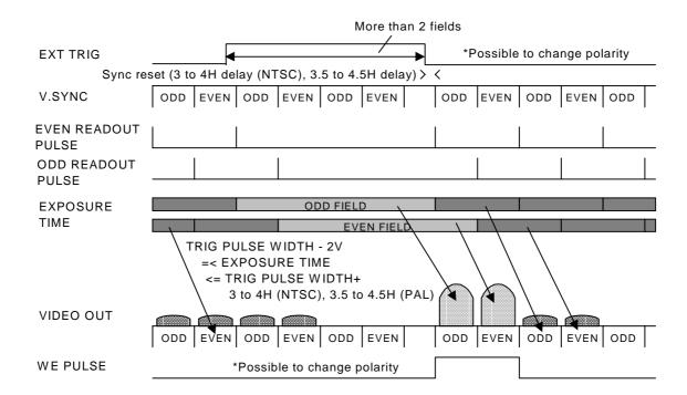
Note: For each external trigger mode, when the end edge of external trigger pulse is input in the timing period when it showed to the under figure, the picture is not output after the SYNC reset. Please input the repetition period of trigger pulse with the following specification, to avoid the trigger input to an above prohibition period.
