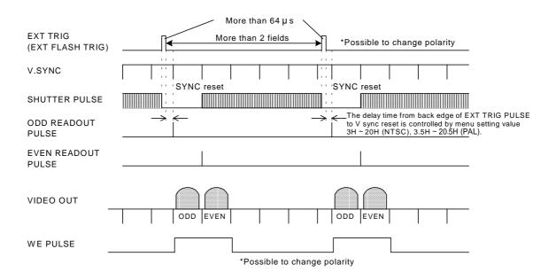
Note: When the flashlight is not used, the even and odd video signal levels are difference as shown to the following timing chart.
