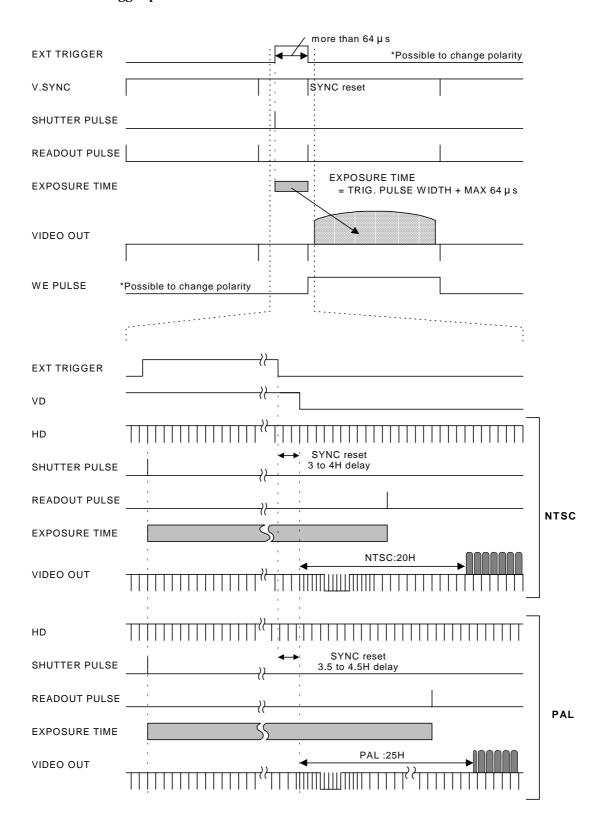
2) Frame on demand (SHUTTER: EXT TRIG, EXT TRIG: MODE1, CCD MODE: FRAME)
